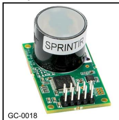
Figura 11: Sensor SprintIR®-W 100% CO 2 - Modelo GC-0018.
